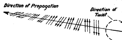
Fig. 6.—Due to the earth's magnetic field a wireless wave slowly rotates in travelling from point to point.
